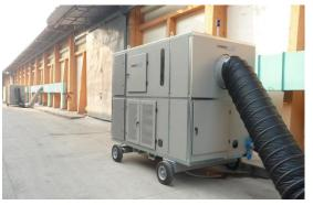
The CONSERFRIO® system, which is based on the refrigeration of the grain in hygrometric equilibrium with it, minimize the mentioned problems and stands for the cleanest, safest and most natural and ecologic method for conserving grains, seeds and most kinds of perishable granulated products.
