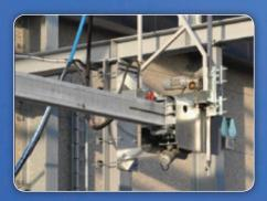
The straight vertical stroke of its probe provides precision and a high force of penetration. The movement is assisted by a variable frequency drive allowing the probe to dive as deep as 4 m even into high density products and powdery material.
